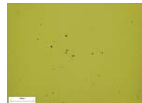
Large Globular Oxides (inclusions) associated with early fatigue failure - seen at 100x magnification of a typical "investment cast" femoral stem
