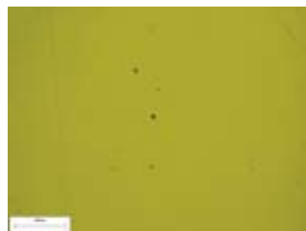
Large Globular Oxides (inclusions) associated with early fatigue failure - seen at 100x magnification of a typical "investment cast" femoral stem
